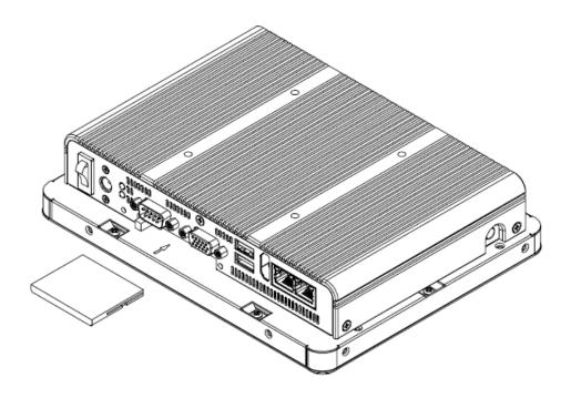
Step 2. Put the CF card into the socket and fasten 2 screws back.
