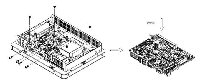
**Step 2.** Unlock 4 coppers from the rear I/O of VGA & COM ports.
