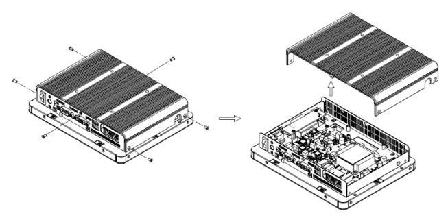
**Step 1.** Unfasten 6 screws to remove the bottom chassis.
