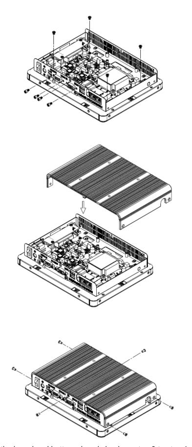
**Step 4.** Assemble the board and bottom chassis back as step 3 to step 1.
