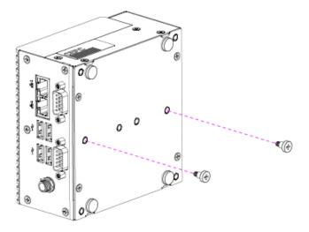
**Step1.** Insert and fasten two screws on the bottom.
