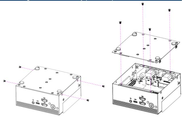
Step1. For HDD installation, remove 8 screws from bottom cover and take it off.
