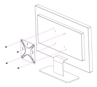
**Step2.** Fix with four screws on the monitor.
