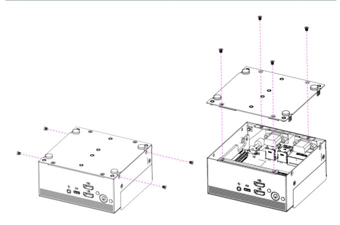
Step1. Remove 8 screws from bottom cover and take it off.
