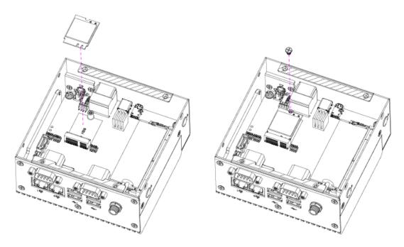
**Step2.** Insert M.2 E-Key (2230) card into designated locations and fasten with screw to complete installation.
