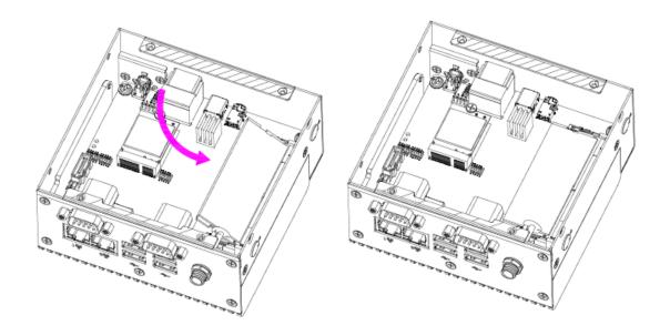
Step4. Slide the DDR5 SODIMM into the memory socket and press it down until properly seated.
