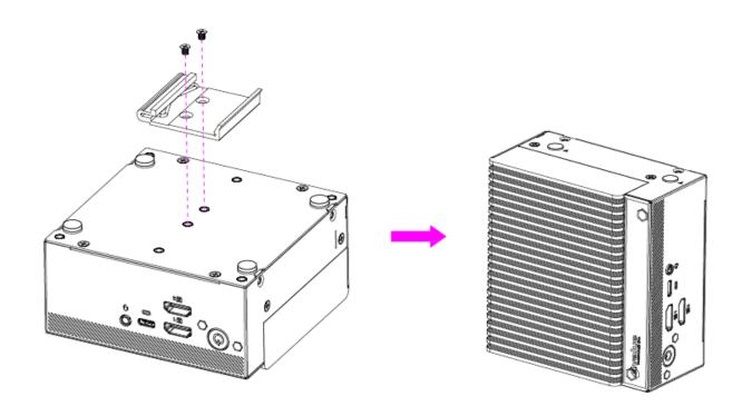
**Step1.** Fix with two screws on the system.
