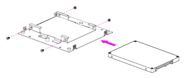
Step2. Install HDD.
