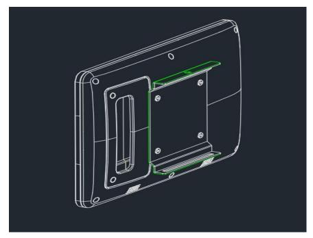
Step1. Insert and fasten 4 screws on each side of VNS-10WAD to secure VESA Mount.
