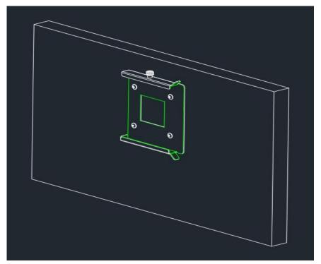
**Step2.** Insert and fasten 4 screws on each side of the monitor to secure VESA Mount.
