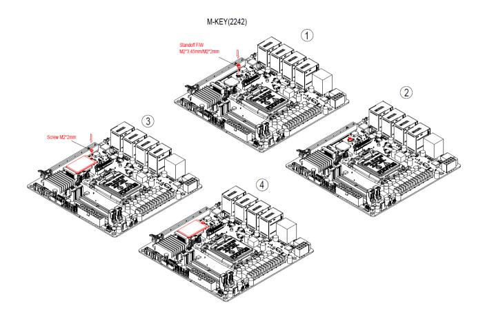
Step1. Insert M.2 M-Key (2242) card into designated locations and fasten with screw to complete installation.
