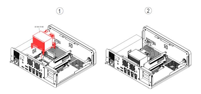
**Step1.** Using 3 screws to lock CPU Cooler through screw holes from the system.
