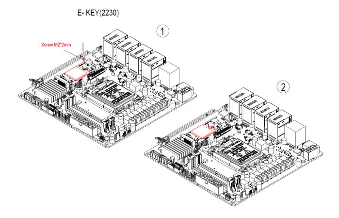
Step1. Insert M.2 E-Key (2230) card into designated locations and fasten with screw to complete installation.
