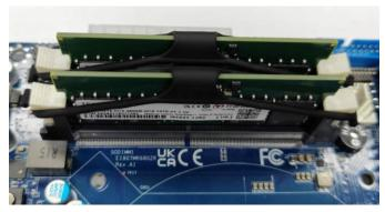
**Step1.** Use a tool to gently lift the straps over the RAM modules.
