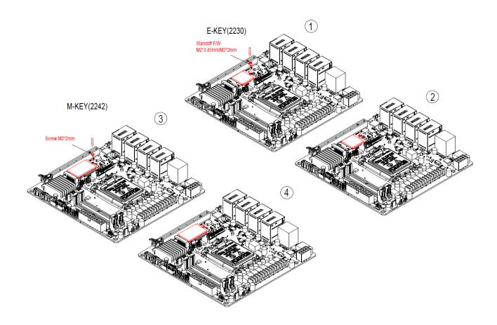
Step1. Insert M.2 E-Key (2230) card and M.2 M-Key (2242) card into designated locations and fasten with screws to complete installation.
