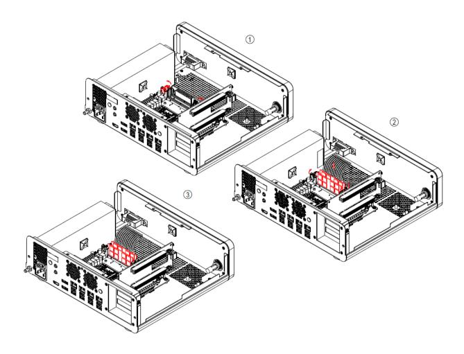
**Step5.** Slide the DDR5 SODIMMs into the memory sockets and press it down until properly seated.
