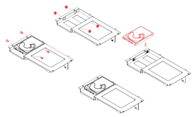
Step3. Secure HDD by means of 4 screws (M3\*8) and 4 shockproof rubbers.
