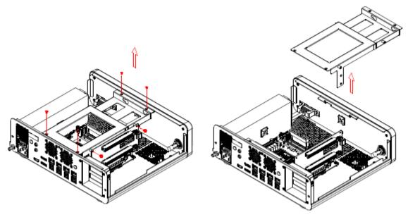
Step2. Remove 6 screws to release the SSD bracket.
