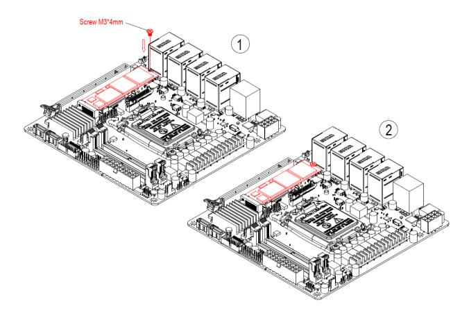
Step1. Insert M.2 M-Key (2280) card into designated locations and fasten with screw to complete installation.
