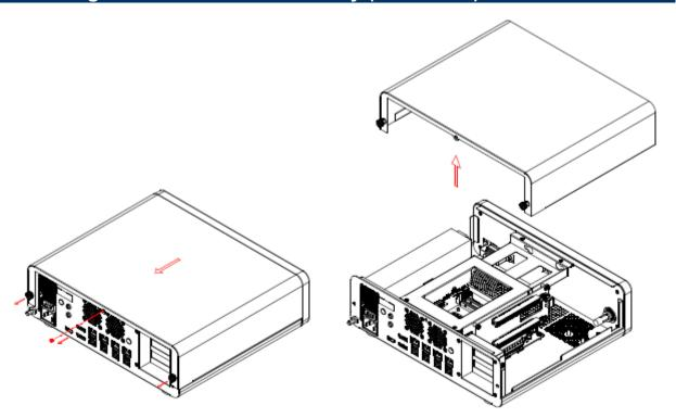
Step1. Loosen the screws on both sides and remove the screw in the middle to take off the top cover.
