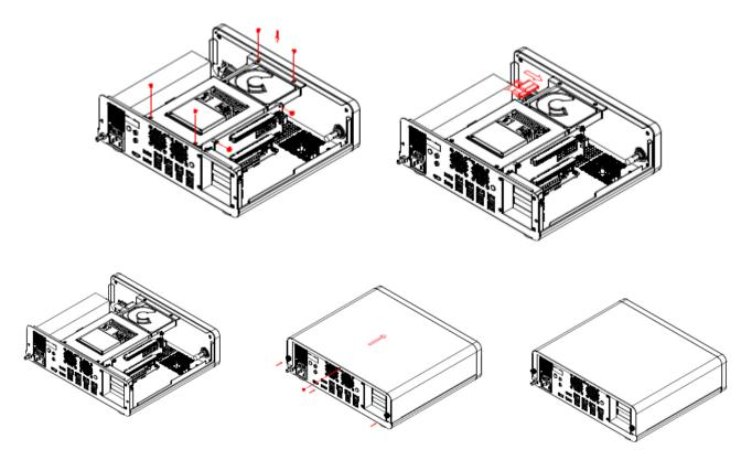
Step4. Insert SSD bracket into designated locations and fasten with 6 screws to complete SSD installation.
